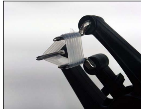
FIGURE 9 - SHROUD STRETCHED WITH TOOL
