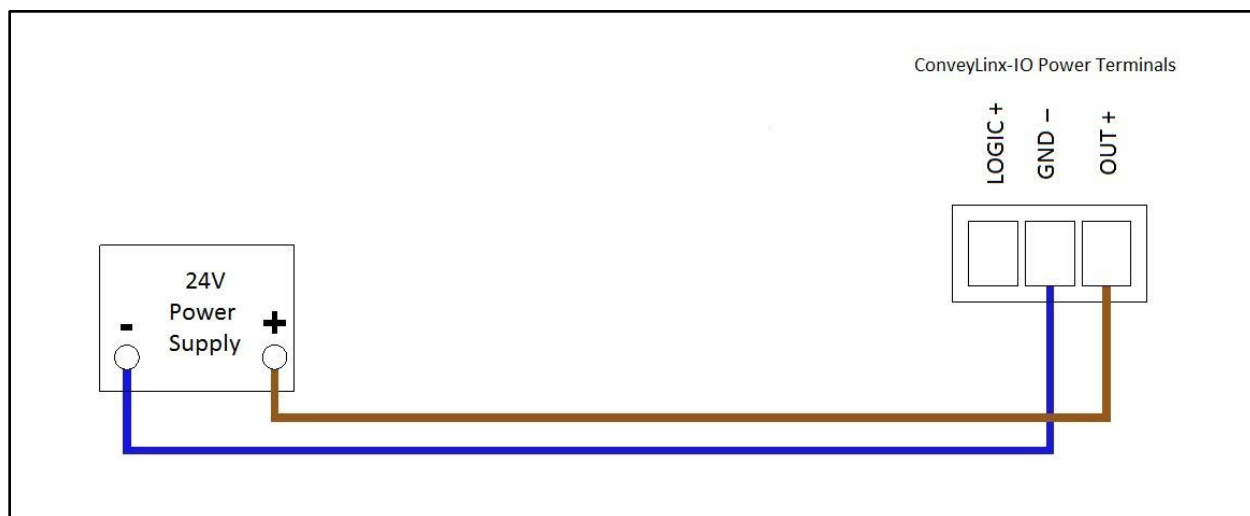
FIGURE 12 - CONNECTION FOR SINGLE OUTPUTS AND LOGIC POWER SUPPLY
