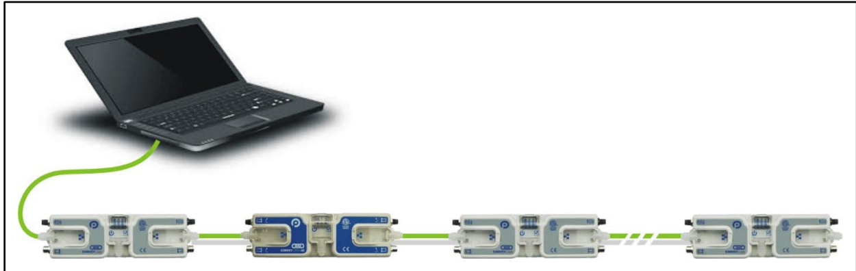
FIGURE 18 - INITIAL PC CONNECTION TO CONVEYLINX SUBNET
